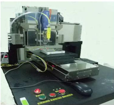
Linear motor submicron stage for optical fiber alignment
